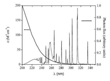
Figure 1: Medium pressure (MP) lamp spectrum (black line) against the adsorption of hydrogen peroxide (bold black line).
