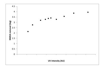
Figure 2: Results of HOD UV AOP degradation of NDMA from an initial concentration of 10,000 ppt to below a discharge detection limit of 2 ppt at a pilot site in North America.
