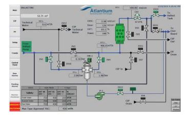
Operators select the Authority (IMO or USCG) for intended location of de-ballasting and the holding time. Then the ballasting or de-ballasting process is selected. The One-Pass™ ballasting mode can also be selected at this time if desired.
