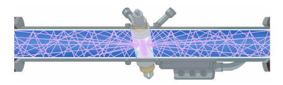
The HOD™ UV system's TIR technology recycles UV light within the chamber to ensure homogenous UV dose distribution while exhibiting superior power (kW) efficiency.
