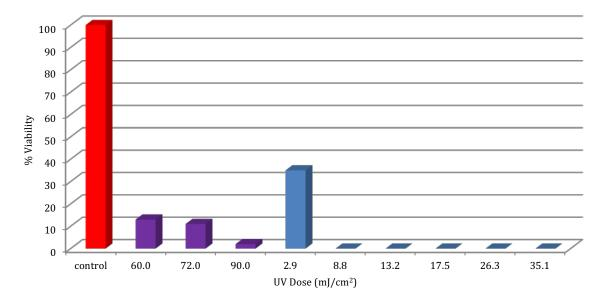
Figure 1: Immediate counting (0h) after UV treatment showed only 22% viability after illumination with the LP lamp at UV dose of 90 mJ/cm<sup>2</sup>, while 100% mortality was observed after illumination with the MP HOD UV lamp at 26.3 mJ/cm<sup>2</sup>.
