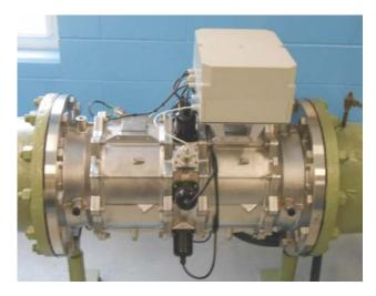
The system uses a proprietary Total Internal Reflection (TIR) based design that when coupled with the comprehensive monitoring of critical parameters allows the system to achieve and maintain the specified UV dose.
