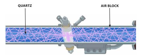
Figure 1: Atlantium Hydro-Optic™ UV Lamp and Chamber
